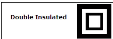
This type of tool will only have a two prong plug. If the tool doesn't state that it is double insulated, then you must have a third prong on the plug. This third prong, or ground prong,
