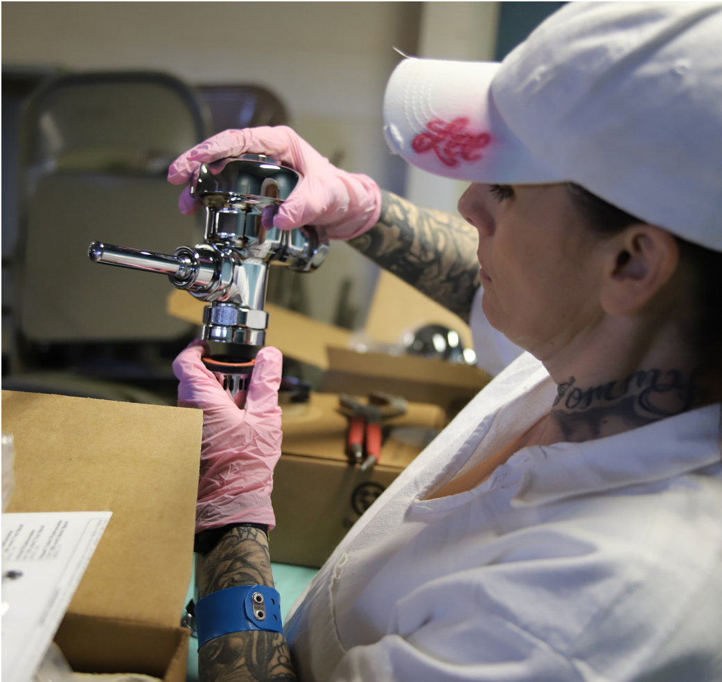
Preceding page: Monica Owens and Amy Lee moving around different housing areas at the Hobby Unit in Marlin; Above: Working on toilets at the Hobby Unit gym; Right: Amy Lee reassembling a flushing mechanism.
